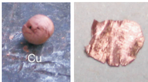
Fig. 4 Bead obtained from malachite by chemical reactions before and after hammering
